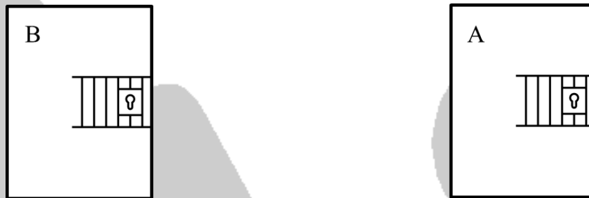
Figure 1-3 The view of the junction boxes from behind the control panel. The instrument technician was required to unlock the junction box to access the signal wire to the recorder-controller. No labels were on the rear faces of the junction boxes—the letters B and A are noted to let the reader know that from the perspective of the technician from behind the control panel, the B junction box is on the left and the A junction box is on the technician's right.
