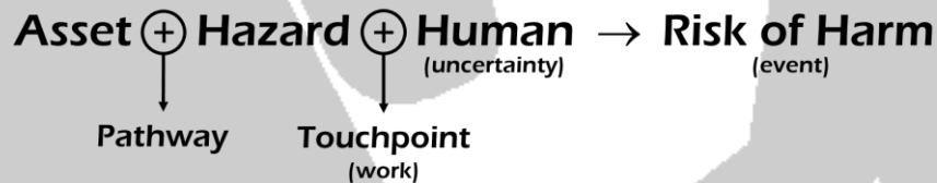
Figure 2-2 The Hu Risk Management Model pinpoints the two work-related interfaces—pathways and touchpoints (denoted by the plus (+) signs)—that must be controlled to minimize the risk of harm during operations. (See Muschara, T. (2018). Risk-Based Thinking (p.30).).
